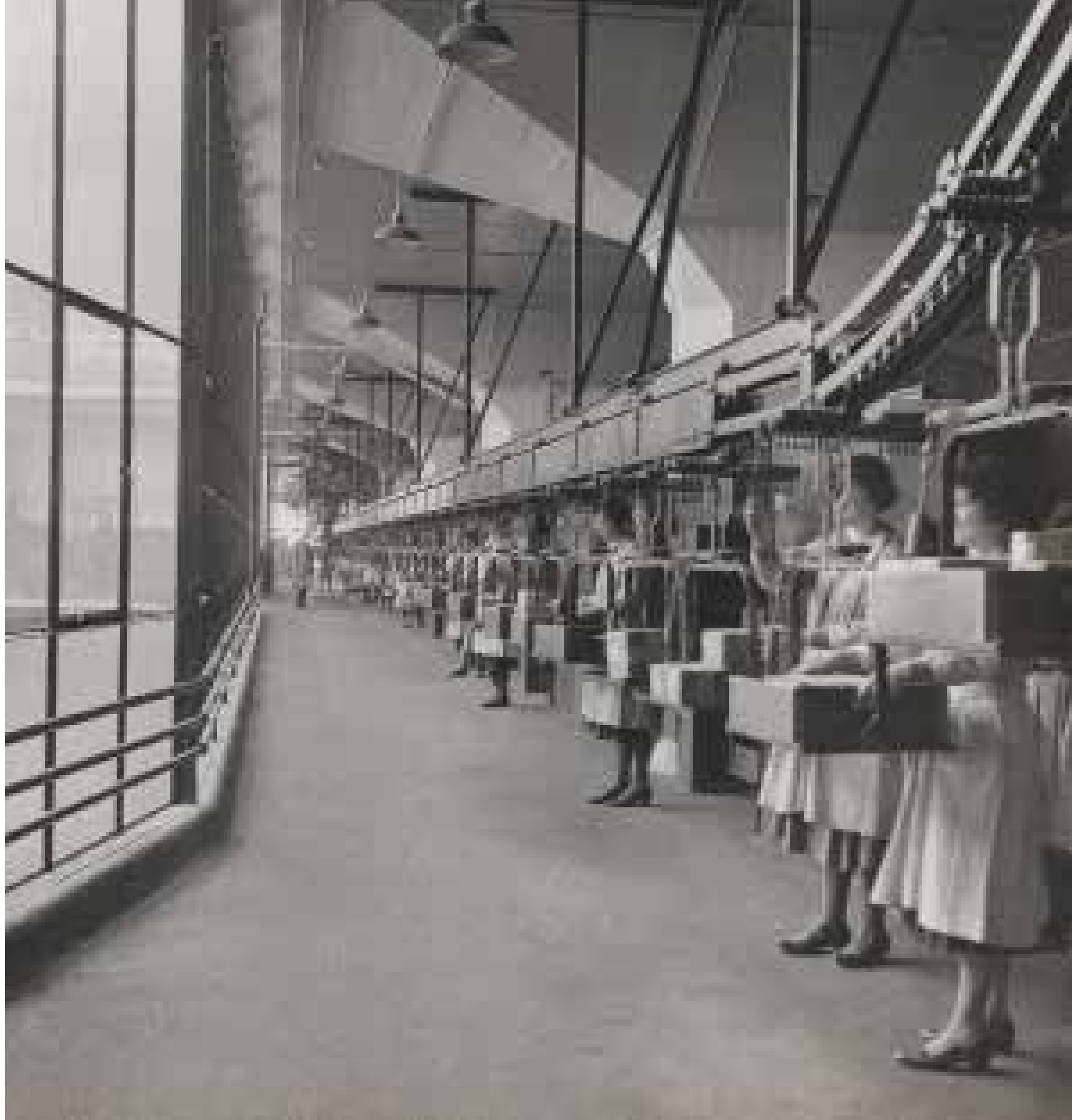
Left: the north side of the Boots D10 factory, near the dispatch loading bay. The jagged spurs were designed to connect to a possible extension, while the projecting rails supported window-cleaning equipment. Right: Women packing boxes on to the overhead conveyor in D10 (c.1935) – notice the male overseer. The horizontal conveyor system was removed prior to listing in 1971
