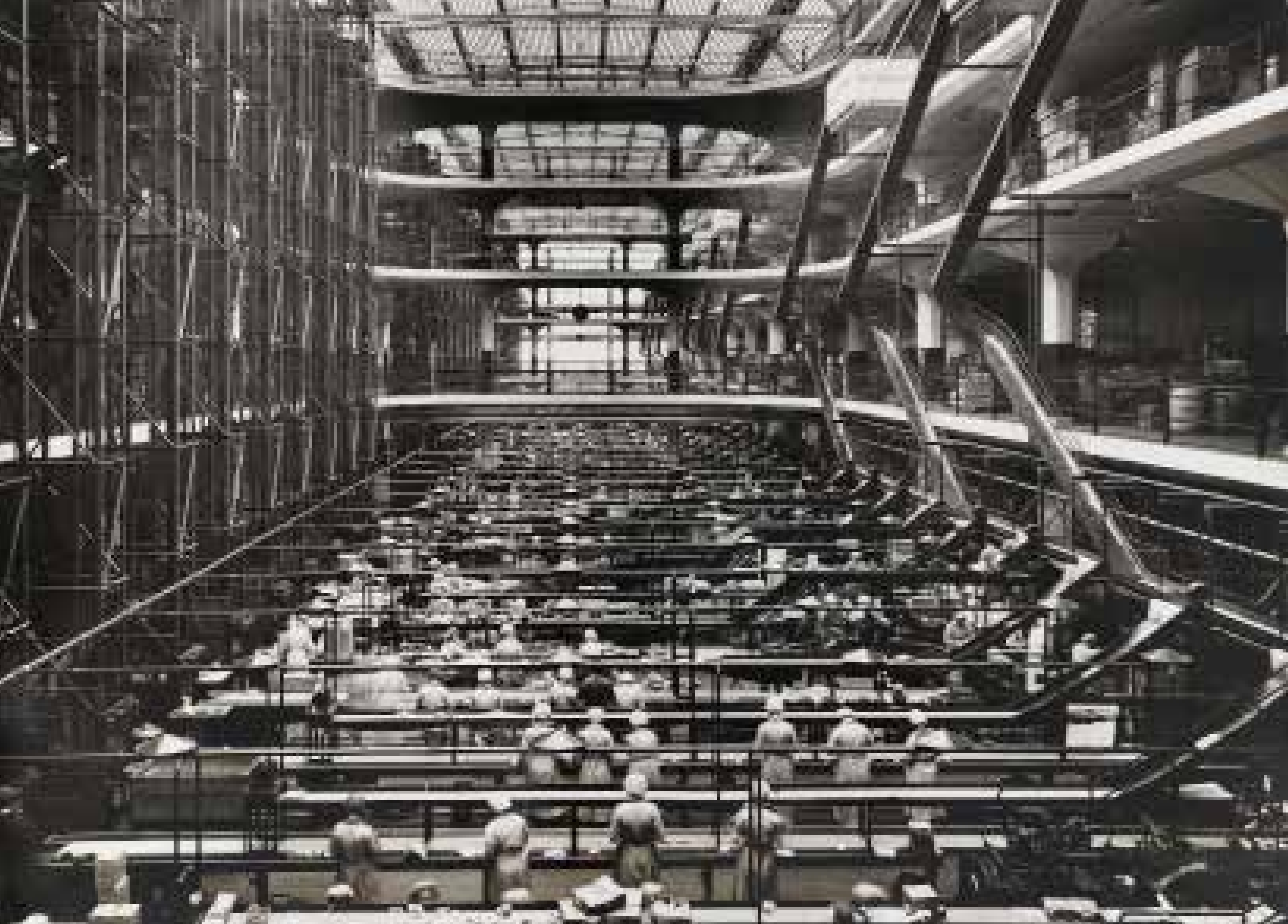
This photograph shows the packing hall looking east, with gravity chutes from the materials store on the right, and vertical hoists to the finished goods store on the left. The overall effect is very similar to Albert Kahn's multi-storey Ford factory buildings of 1914. Kahn, with his brothers Julius and Moritz, set up the Trussed Concrete Steel Company (Truscon) and opened a London office in 1907. Williams worked there from 1912-16. But by the time D10 was complete, the American car industry was moving towards single-storey factories
